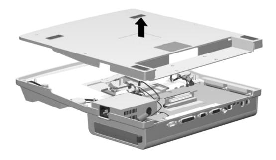
Figure 6-10. Removing the Bottom Cover Assembly
